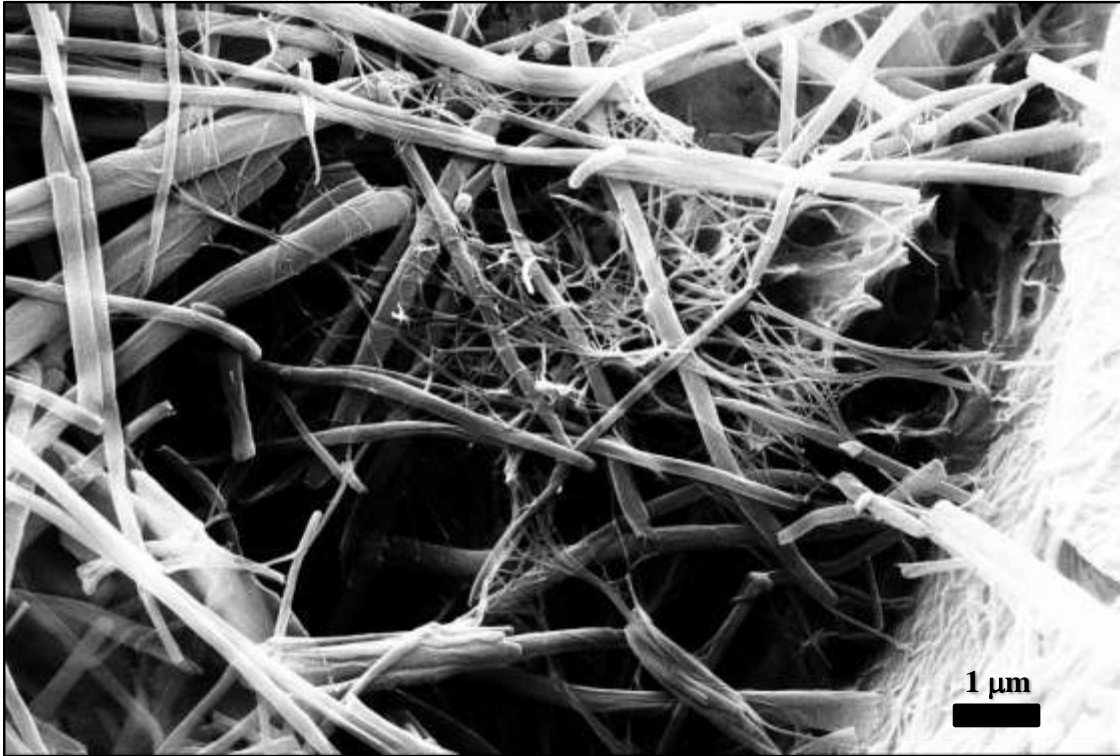
Figure 2.17 - Typical dispersion state of s-MWCNTs in mortar matrix at 1%
