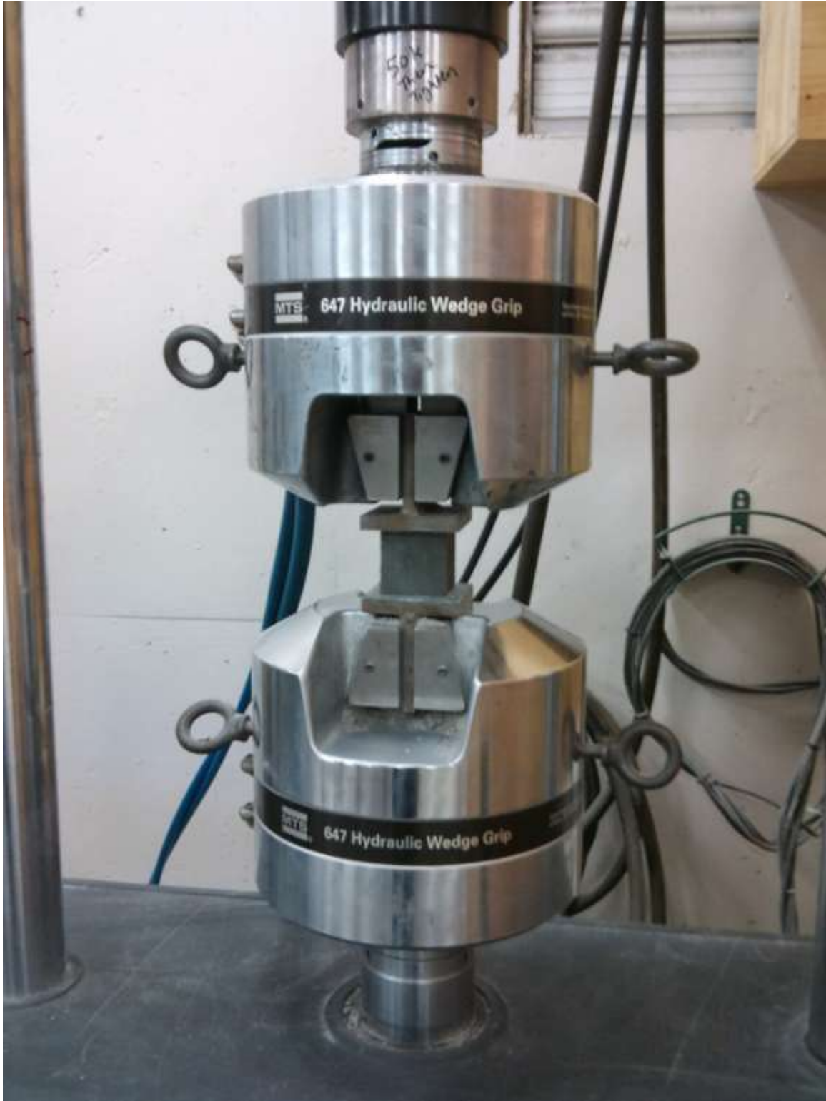
Figure 2.3 - Compression tests setup – Tests were performed in displacement control using a 810 MTS Material Testing System
